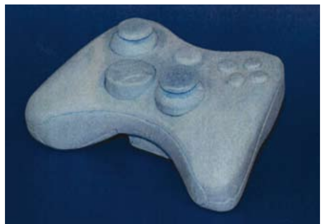
Figure 1.12 A student's Styrofoam™ model of the games controller used in the product investigation task.
