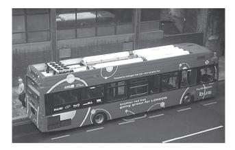
The bus uses hydrogen as a fuel. There are six hydrogen fuel tanks, which can be seen on the roof of the bus. The hydrogen from the tanks reacts with oxygen from the air in a fuel cell to release energy to power the bus.
